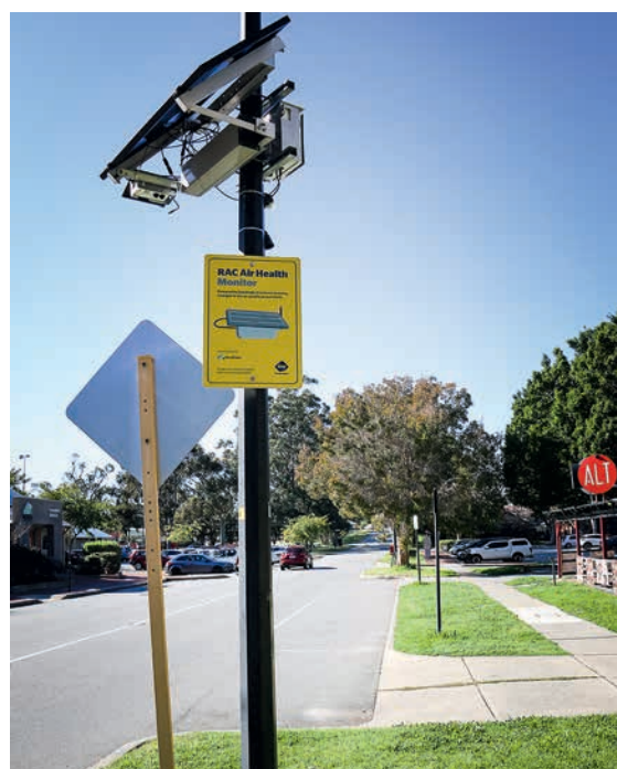
▲ RAC Air Health Monitor sensor and black carbon module with community signage
