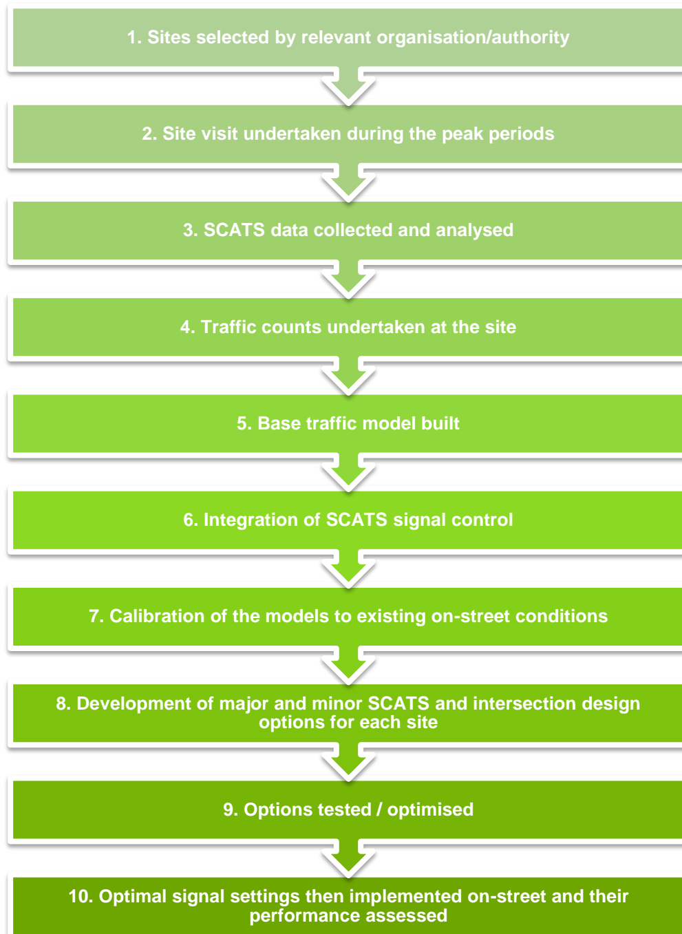
Figure 8-2: Signal adjustment process used for this study
